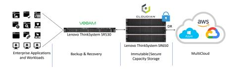
Lenovo Object Storage Powered by Cloudian provides a fast, on-prem, capacity-tier storage target for Veeam Availability Suite deployed on Lenovo ThinkSystem Servers. The Object Lock feature ensures protection from ransomware.
